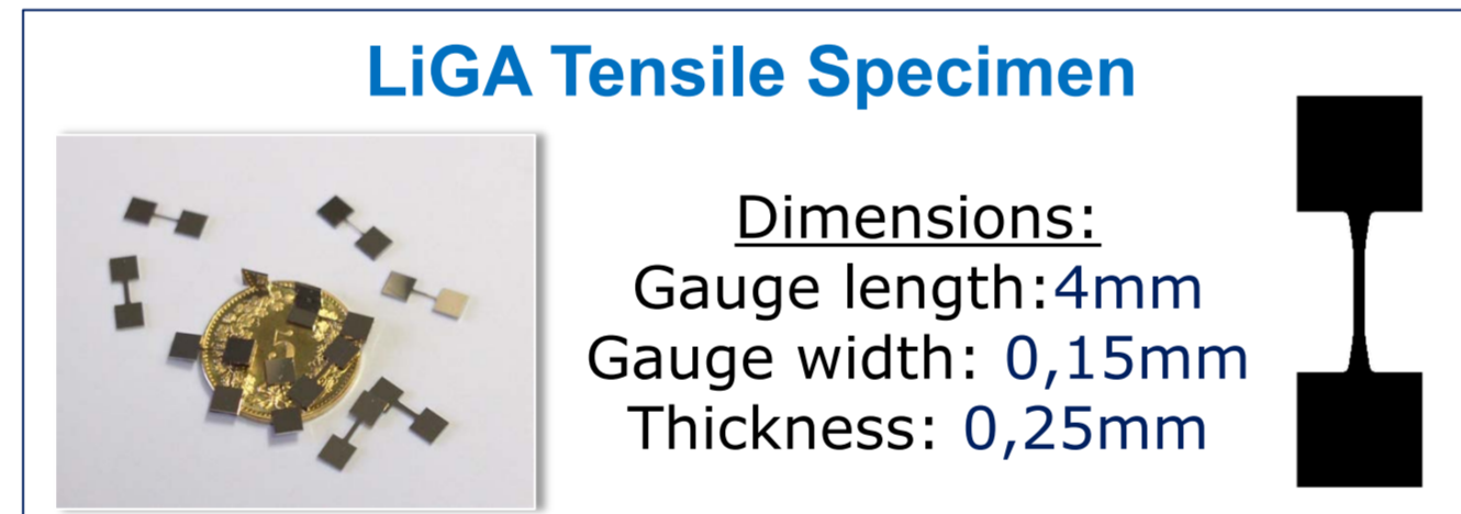
Above: LiGA micro specimen dimensions Left: In-Situ tensile stage (Kammrath & Weiss) with modified displacement sensors, load cell and gripping system
