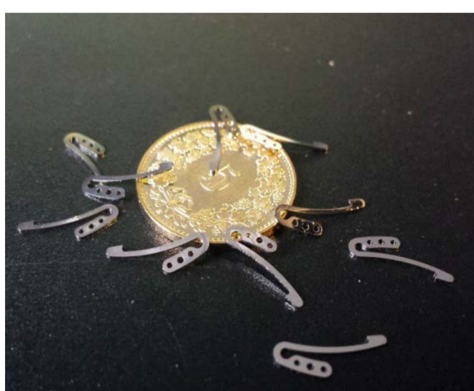
Ni micro components, deposited into LiGA-mold
