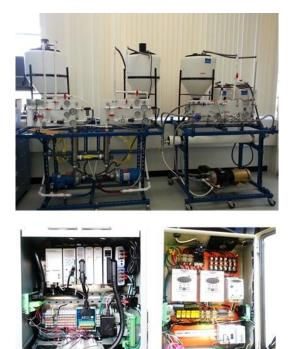
Figure 1 – A pilot scale FORO plant (top image) with a PLC based data acquisition system (bottom image)
