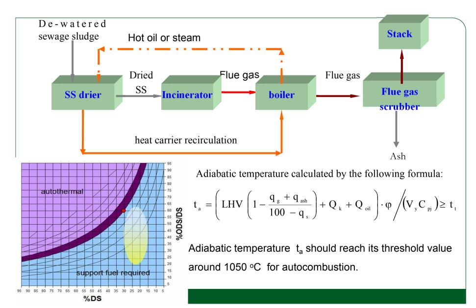
SS can be burnt in the coal-fired boilers, MSW incinerators and incinerated independently. For comparison, the commonly used fluidized-bed drying & incineration alone is adopted here:
