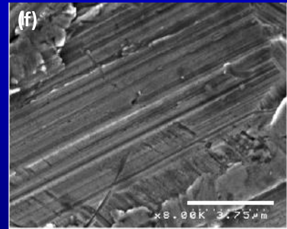
SEM images of the Ti surfaces coated with (a) 170 nm, (b) 150 nm, (c) 130 nm, (d) 110 nm hydroxyapatite powders, (e) plasma sprayed micron sized hydroxyapatite onto Ti and (f) plain Ti. Scale bar: 1 micrometer
