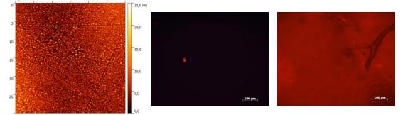
Figure 1 - AFM image of a PVCL/MEA 20 microgel film (left), fluorescence microscopy image of a PVCL/MEA 20 microgel film after incubation with tetramethylrhodamine-BSA (middle) and pure glass after incubation with tetramethylrhodamine-BSA as reference (right).
