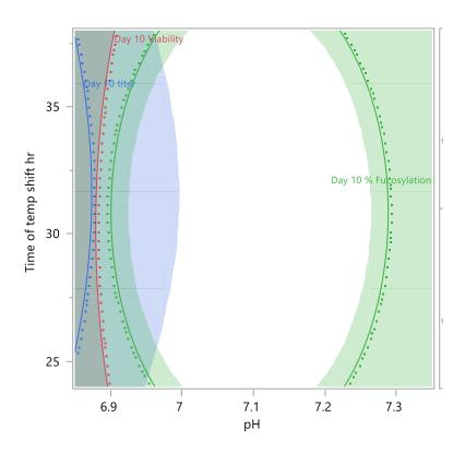
Figure 1 – Design space for critical process parameters satisfying the critical quality attributes of an IgG
