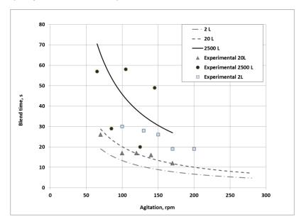
Figure 1 – Blend time design chart and experimental data for different bioreactor scales
