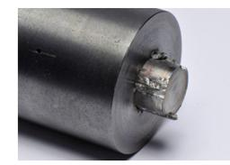
Strong adhesion of punch and die during SPS at 400°C
