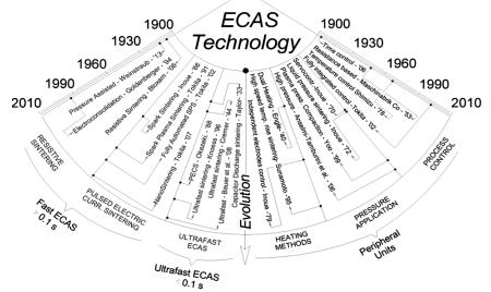
**Fig. 1** Diagram tracing the evolution of ECAS technology over the past 110 years. The main patents corresponding to milestones in basic ECAS and peripheral units, are specified on the left- and right-hand sides, respectively.
