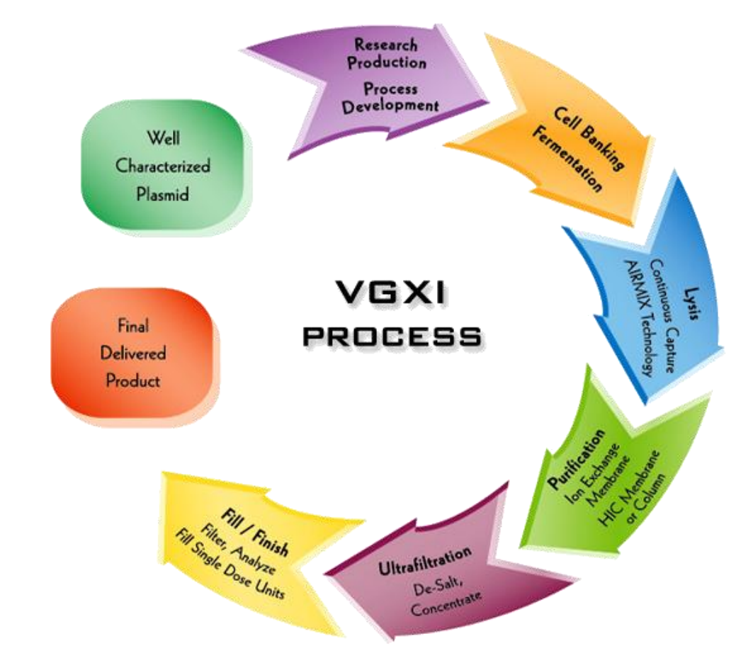
Figure 3. Schematic of the VGXI manufacturing process from receipt of a client plasmid through cGMP delivery of filled vials.
