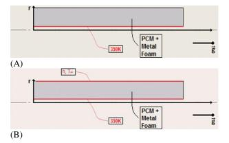
Figure 2: THE TWO CONFIGURATIONS WITH DIFFERENT BOUNDARY CONDITIONS FOR THE OUTER SURFACE: (A) ADIABATIC AND (B) CONVECTIVE HEAT TRANSFER.
