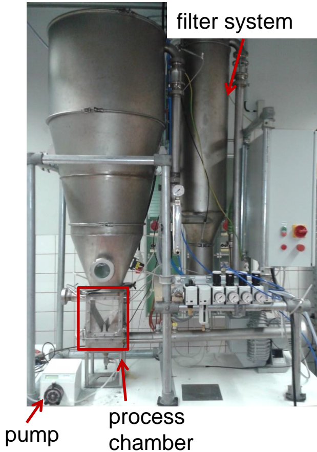
spouted bed apparatus optimized for fine particles
