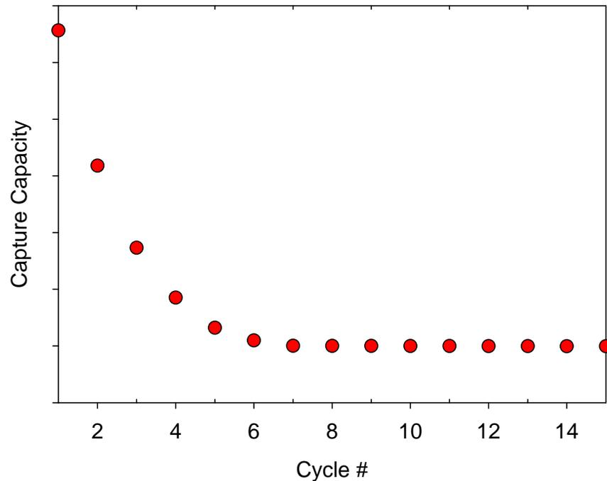
Decay of CO<sub>2</sub> Capture Capacity
