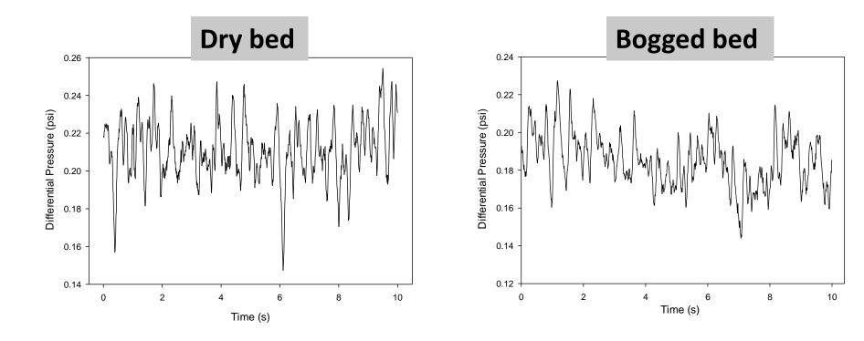
Differential pressure data measured between two vertically separated pressure taps for  $U_f = 0.1 \text{ m/s}$
