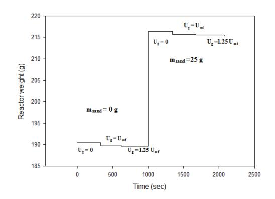
The variation of the reactor weight was the same for different initial weights of the bed of 0 g and 25 g
