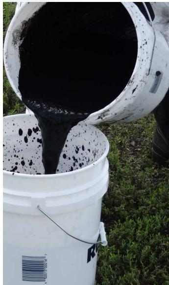
Example of Sorel-Tracy : Before WAO : 20 000 tons of sludges After : 1 400 tons of solid (> 99% inorganic) + biodegradable liquid
