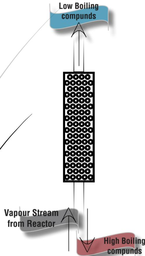
**Fractionating system is a distillation apparatus**
