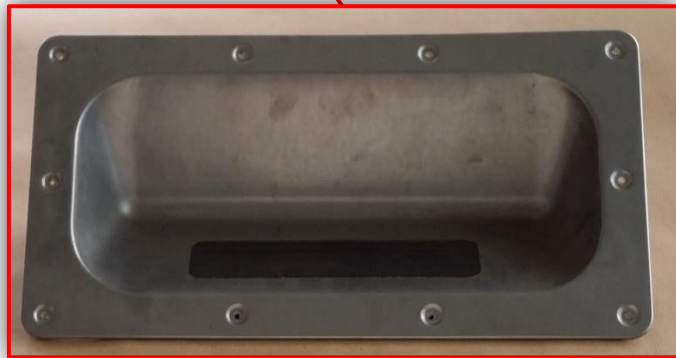
Cargo foot step made of titanium (source: Airbus)
