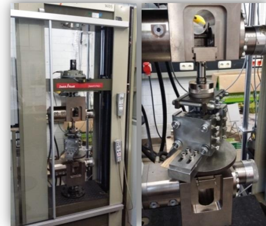
Testing machine and equipment for CAI
