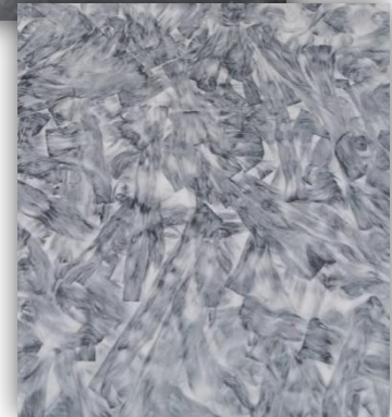
Carbon fibre SMC with UP matrix
