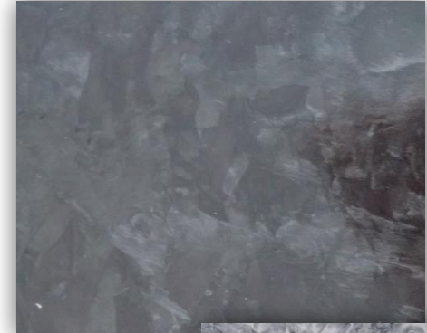
Carbon fibre SMC with EP matrix
