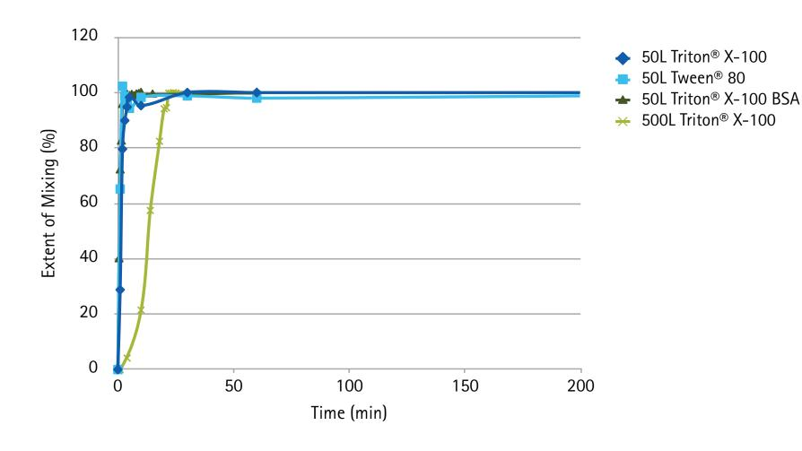
• Mixing essentially completed by 10 min at 50 L; 22 min at 500 L
