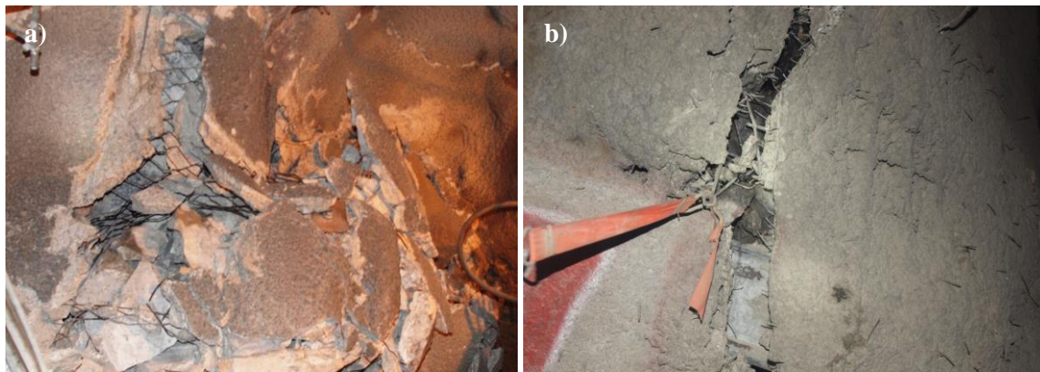
Figure 11 - Post fracture displacement capacity of a) high tensile articulating chain link mesh and b) mild steel weld mesh
