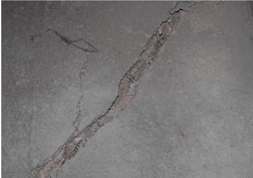
Figure 13 – Encapsulated mesh provides superior post-fracture energy dissipation capacity.
