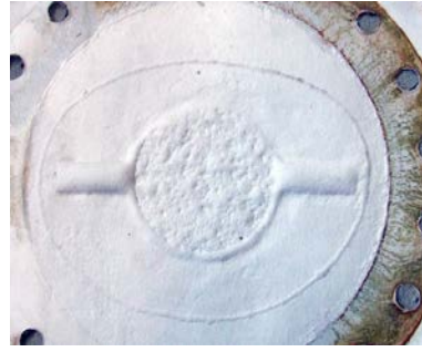
Figure 10. Geotextile after test
