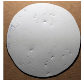
Figure 12. Membrane loaded with 5.0 MPa
