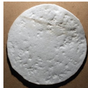
Figure 13. Geotextile loaded with 5.0 MPa
