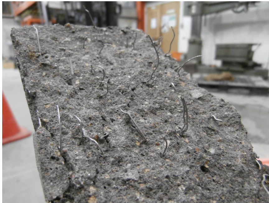
Figure 6: Fracture surface of a RDP test panel; failure involves primarily pull-out of the fibers ( Normal consistency level).
