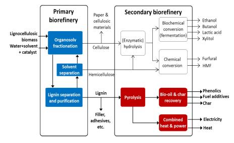
Organosolv comprises an effective fractionation of lignocellulosic biomass into a cellulose pulp, a hemicellulose-rich syrup and a high-purity lignin.
