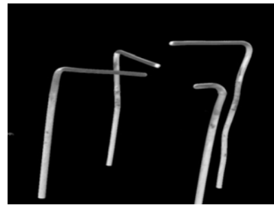
Figure 13. Thermocouple localization through X-Ray Computer tomography
