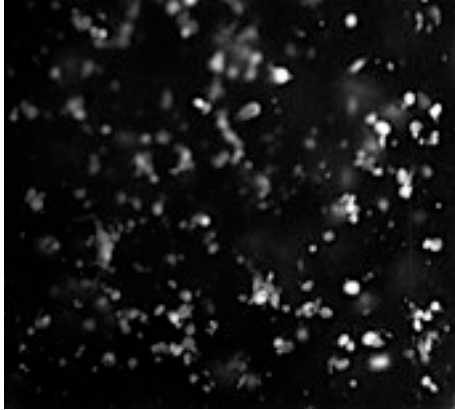
Figure 6: High speed video frame of FCC catalyst in the freeboard region of a 16-cm (6-inch) diameter fluidized bed at a superficial gas velocity of 0.61 m/sec (2 ft/sec). Images were collected at 4000 frames per second with a 20 \mu s exposure time.
