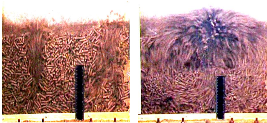
Fig. 3. - The state of straw pellets beds when the air velocity is 2.4 m/s (a) and 3.09 m/s (b).
