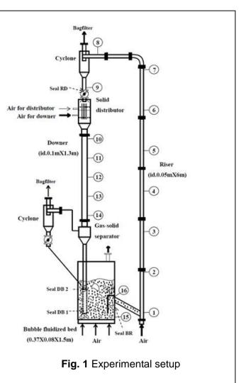
separated with the gas by a quick inertial separator with an efficiency of more than 96% and returned to the BFB. The solids entrained by the gas was further separated by a cyclone and returned to the BFB. The superficial gas velocities of the riser and the downer ranged from 3 to 8 m/s and from 0 to 5 m/s, respectively, but that of BFB was fixed at 0.03 m/s.
