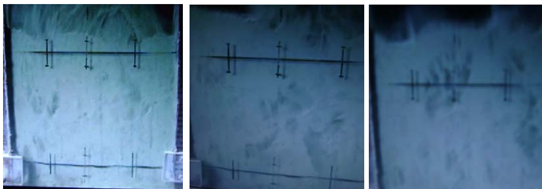
Figure 3. Unique bubble braking phenomena of GSS fluidization
