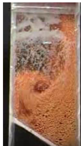
Fig.12 Solid circulation in wetted binary solids fluidized bed with inclined distributor. 7
