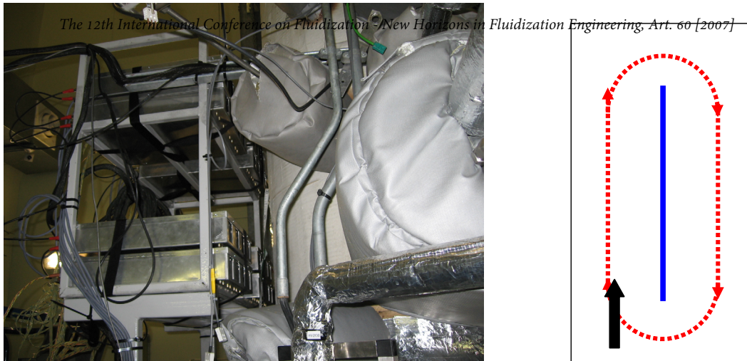
Figure 8: (left) detector arrangement in situ next to lagged bed; (right) circulation arrangement, with central baffle; arrow shows additional gas injection.
