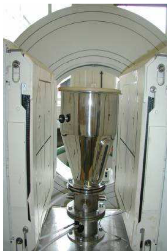
Figure 1: Schematic Diagram of the Wurster Coater (left) and Photograph of Wurster Coater in the PEPT camera (right).
