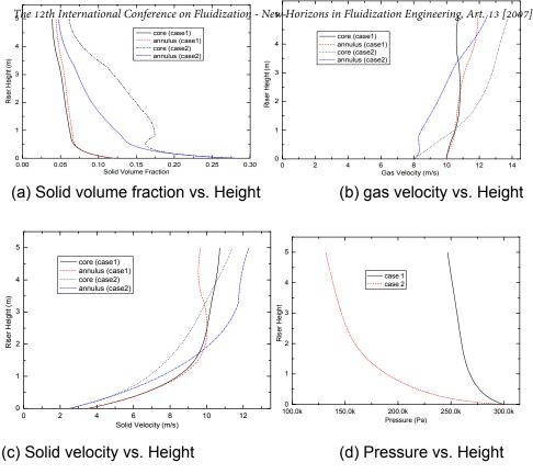
Figure 5 Typical axial distributions of gas-solid flows in riser.
