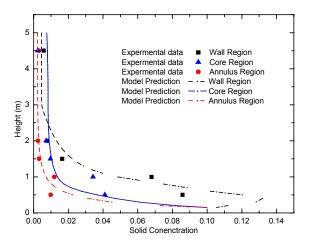
Figure 4 Solid Concentration vs Height
