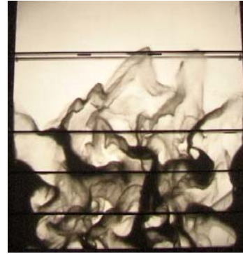
Figure 1. Flow structure at air flow rate 1250 l/min ( U=1.54 \text{ m/s} ).
