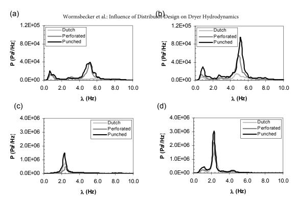
Figure 6: Power Spectrum for 3.0 kg Loadings Dried at 1.5 m/s (a) 16 minutes into drying; (b) 32 minutes into drying; (c) 56 minutes into drying; (d) 88 minutes into drying
