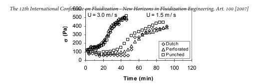
Figure 5: Standard Deviation of Pressure Fluctuations for 3.0 kg Bed Loading
