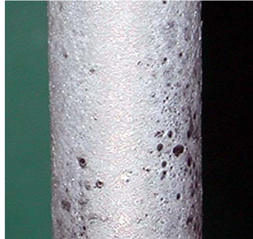
Fig. 8 Whey protein fouling layer
