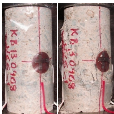
Figure 3. Shotcrete sample before and after UCS test.
