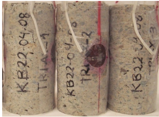
Figure 10. Samples after triaxial test.
