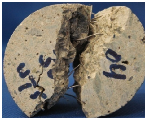
Figure 7. Samples after Brazilian test.
