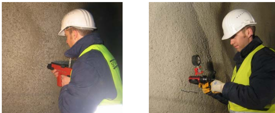
Fig. 2: Determination of early strength using a) bold-driving and b) pull-out device
