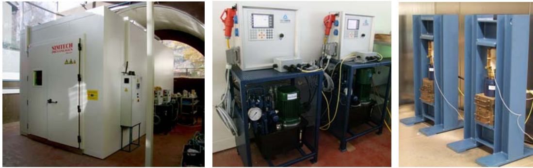
Fig. 9: a) Climate simulation cell with b) hydraulic equipment and c) long-term test rigs
