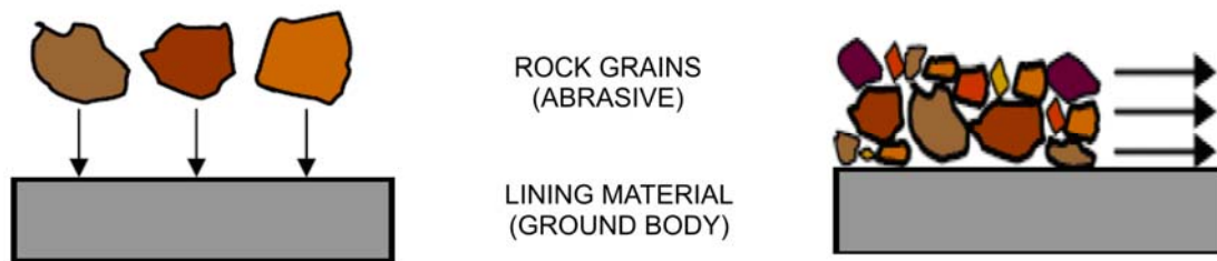
Fig. 14: Types of wear on the lining material
