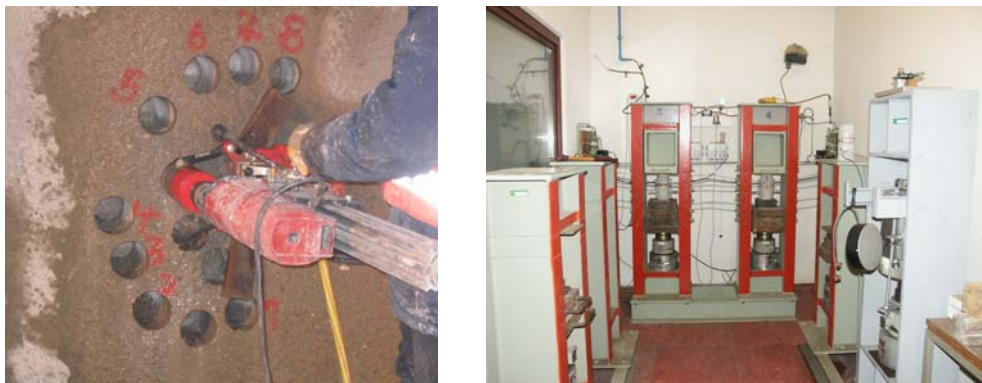
Fig. 6: a) Sampling by coring and b) long-term test rig
