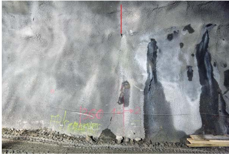
Fig. 13: Area of side wall with local application of polymer-modified sprayed concrete (left) and reference sprayed concrete (right)
