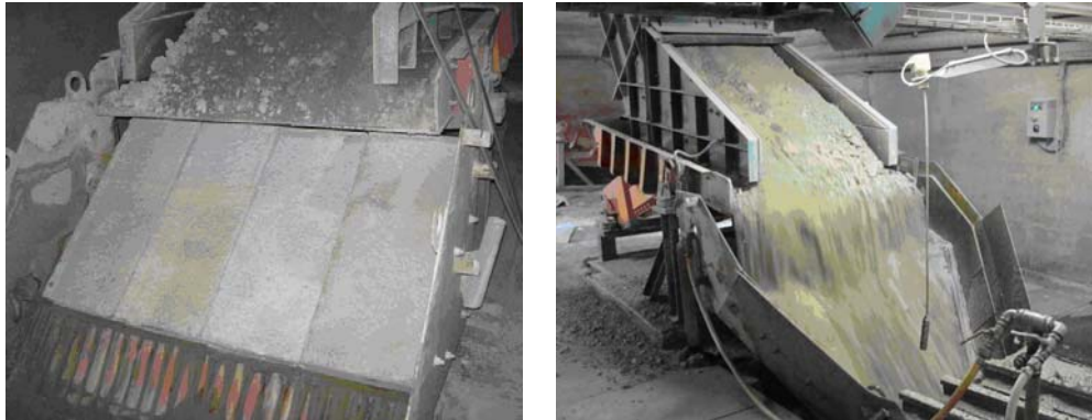
Fig. 18: In-situ tests with test slabs at a material transfer location in the processing plant to investigate the wear behaviour
