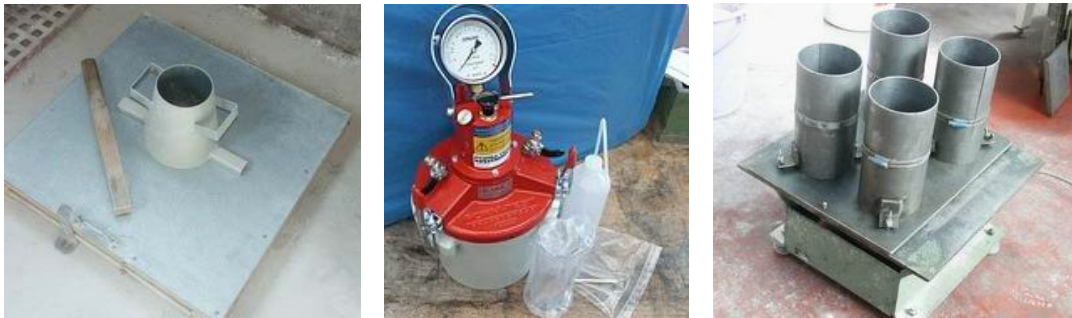
Fig. 1: a) Flow table, b) Air meter c) Cylindrical steel forms
