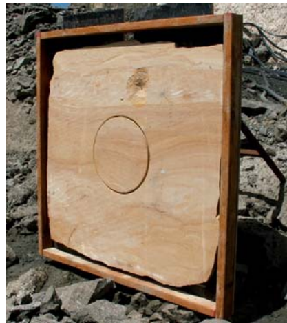
Figure 2: Upright substrate ready for spraying.
