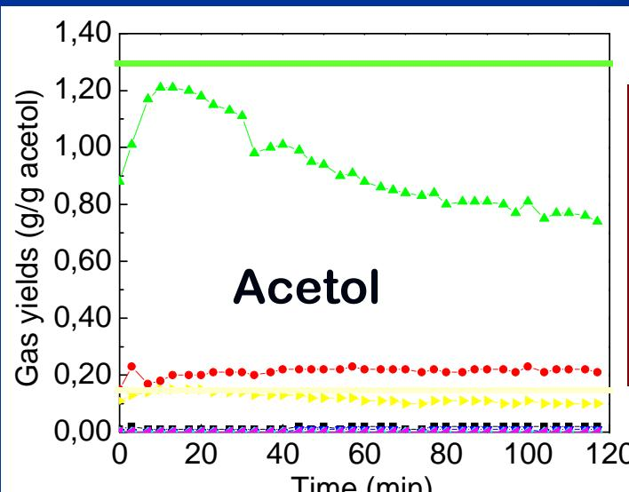
↳ Significant non catalytic reforming for acetol.
