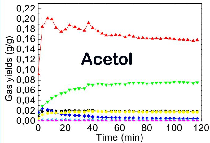
Catalytic Reforming.  $W/m_{org} = 1.46 \text{ g}\cdot\text{min}/\text{g}$ , 650 °C
