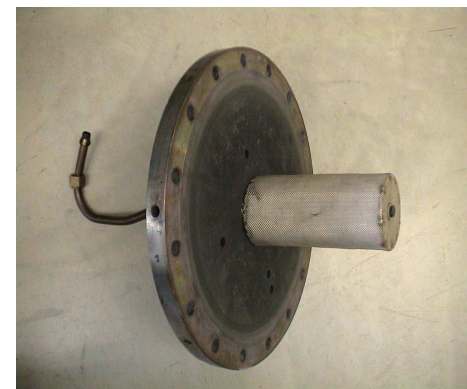
Pilot Plant Reactor Top
