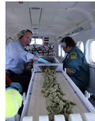
Aerial baiting is done using a bait machine.
