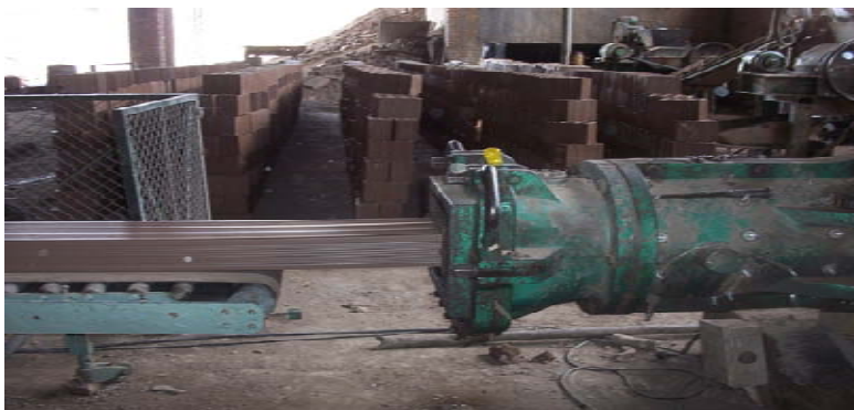
Bricks exit from the extrusion machine and storage previously to introduce in the oven
