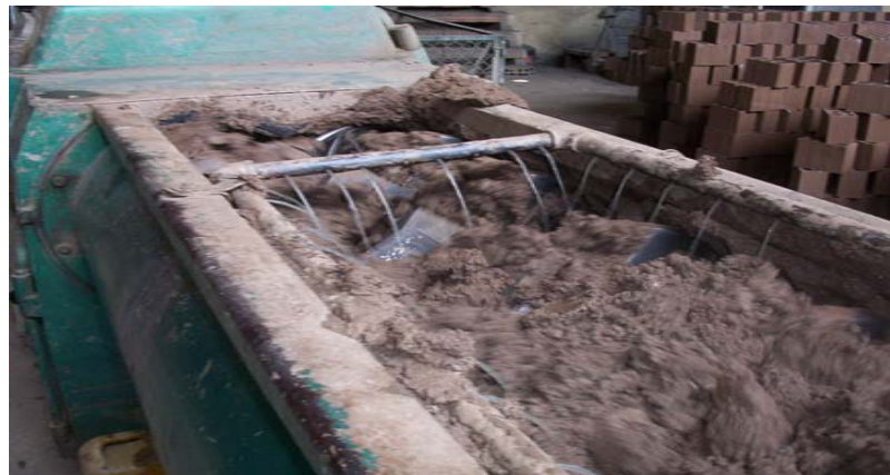
Stages of Clay–Ash mixture and water addition in extrusion machine
