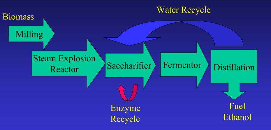
Advantages: fewer solids in reactor, easier to remove inhibitors, higher temp. enzyme rxn.
