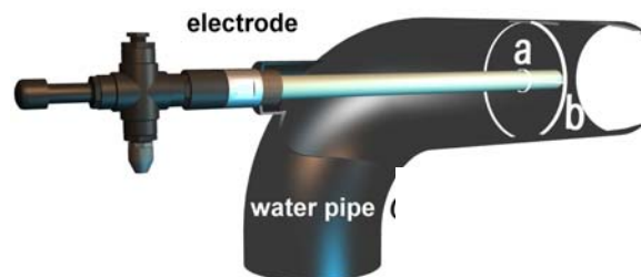
Figure 1: Illustration of the capacitor formed in a pipe by an HVCB System. Courtesy of Zeta Corporation.
