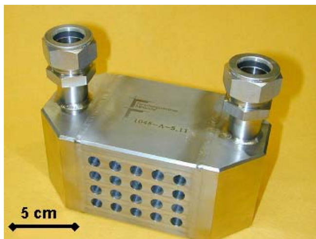
Fig. 8: Electrically powered microchannel heat exchanger used to heat a production mass flow of 1000 kg/h biodiesel.
