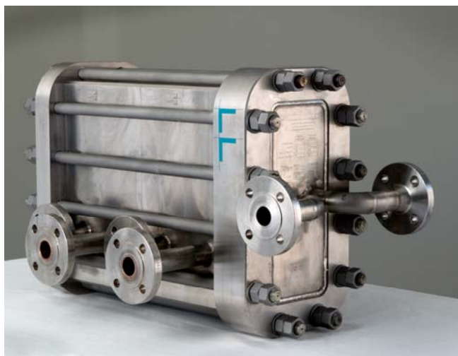
Fig. 9: Microstructure reactor for chemical production. In cooperation with the company of DSM, this device was developed and manufactured. It is about 650 mm long and weighs 290 kg. Several thousand microstructures are integrated to provide excellent mixing and heat transfer.
