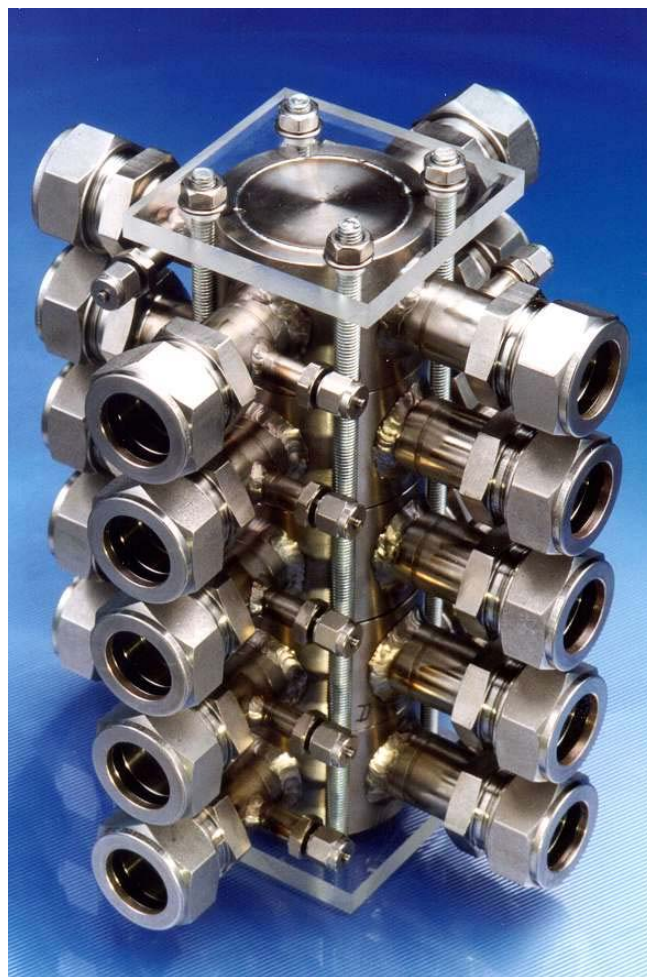
Fig. 7: Stack of five crossflow microchannel heat exchangers. 1 MW thermal power can be transferred at a water mass flow of 35 tons per hour and per passage.
