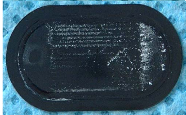
Figure 8: microstructured device and metallic foil (DLC) of the disassembled microstructured heat exchanger.
