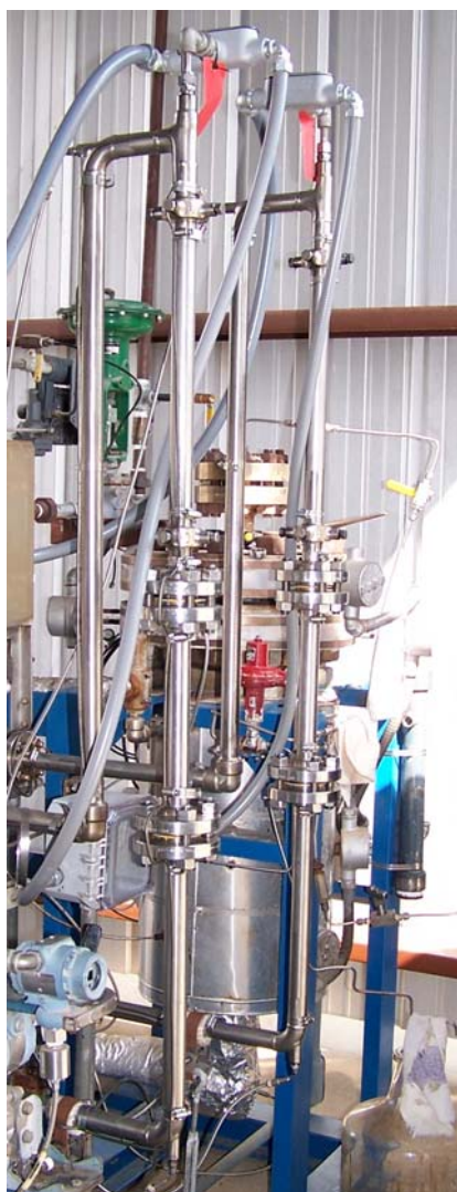
Fig. 3 Photograph of uninsulated HTFU test sections without pressure drop transducers implemented
