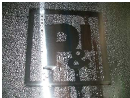
Fig. 11 Photograph of bare Al surface and OPZ treated Al surface after water spraying (symbol of P&I: OPZ treated surface, and other place; bare surface)
