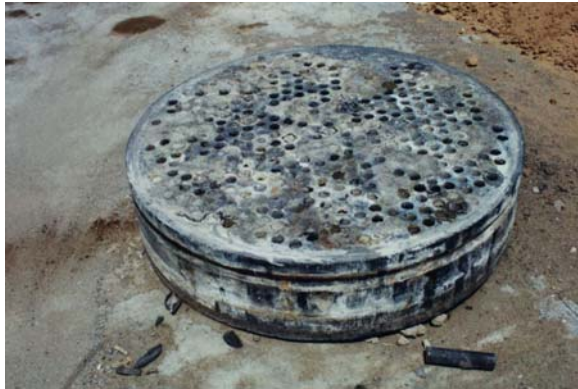
Fig. 2 Deposits on the heat exchanger head
