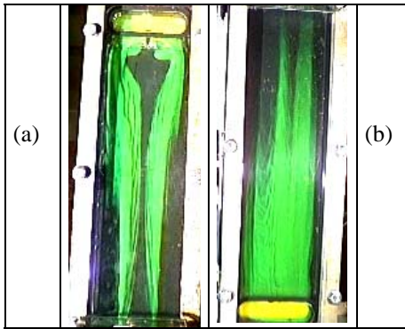
Figure 6: Flow pictures ( Re = 63 ); (a): downward pass with initial inlet geometry; (b): upward pass with modified inlet geometry.
